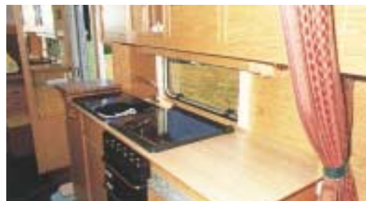
Innocent-looking kitchen (left) conceals such modifications as re-profiled surface edging, removable hob lid, more modern cooker and sink, and perfectly aligned cabinets
