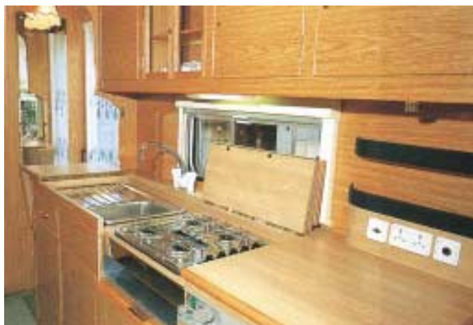
Stainless hob and sink will look familiar, but re-profiled and flush-fitting covers are new
