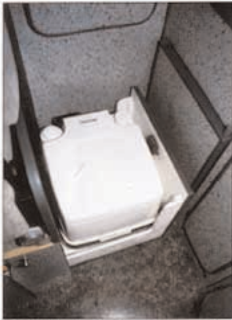
Porta-Potti pulls out into the kitchen area for use
